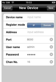
You can select either 'IP' or 'Domain' register mode to login the device, domain mode is for the case that there is no fixed IP address available.
